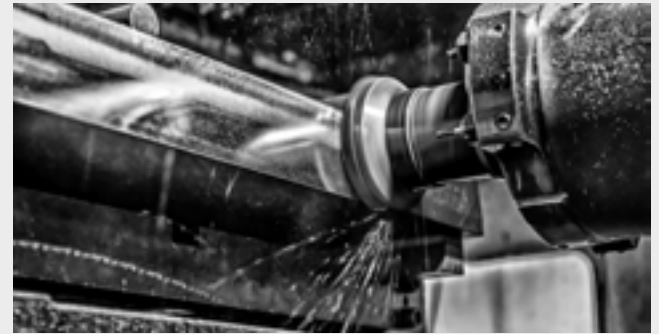
Edge milling of cast iron table
