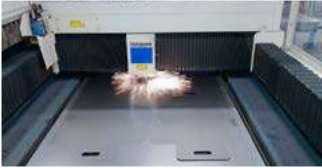
Steel plate laser cutting
