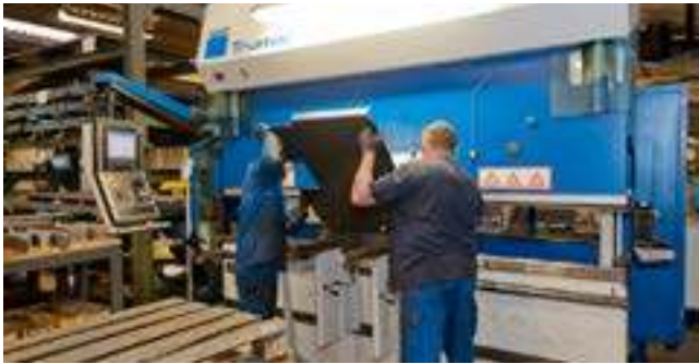
Computer assisted steel plate bending
