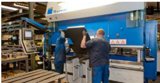
Computer assisted steel plate bending
