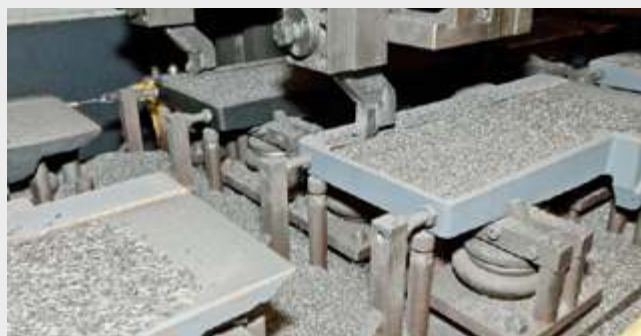
Surface scraping of cast iron table
