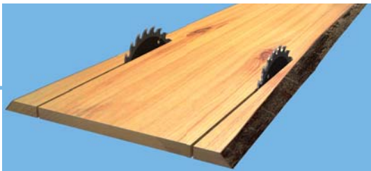
Fig. 23: Board edging in the edger
