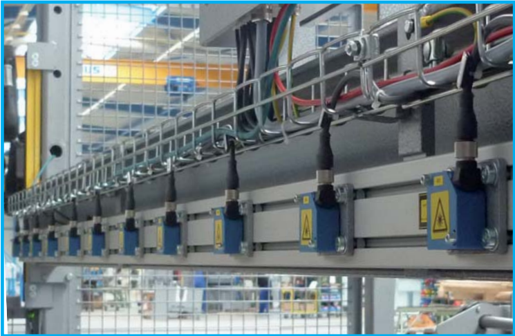
Fig. 4: The measuring heads of the fully automatic AB920 infeed system
