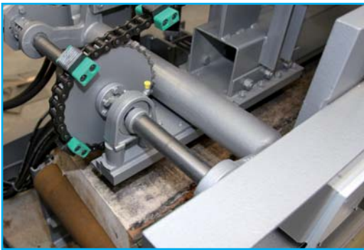
Fig. 8: Bottom rollers and a powered chain above ensure accurate transport into the rip saw
