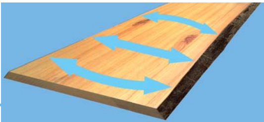
Fig. 22: Measurement and alignment of wane-edged boards in the automatic infeed system
