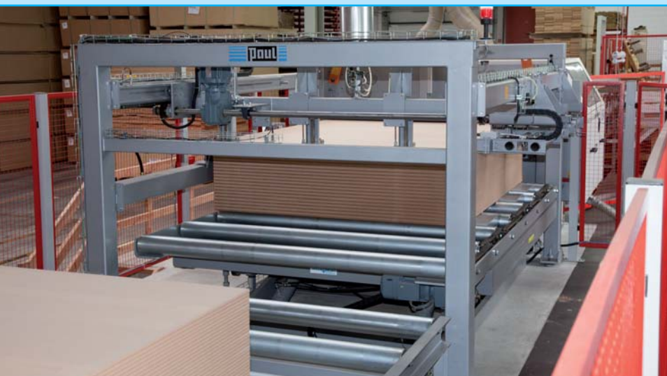
Fig. 27: Multirip saw with automatic feeding system in the production of strips
