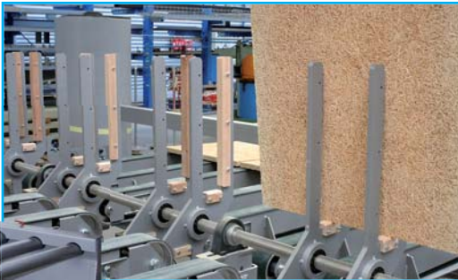
Fig. 23: Automatic panel turn-over device
