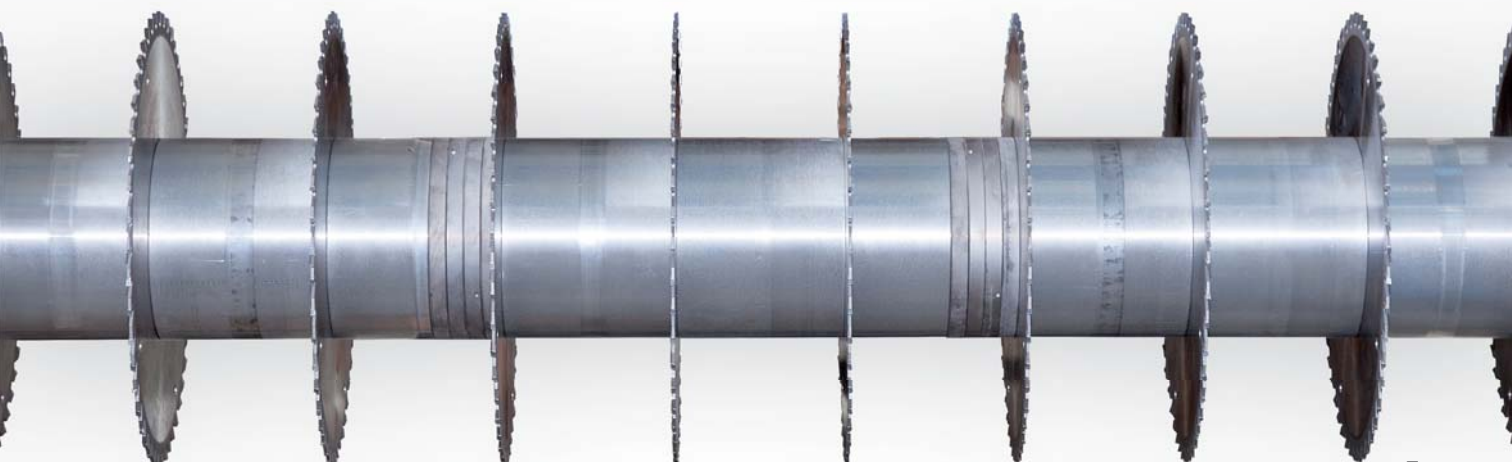
Fig. 12: Saw shaft set up with saw blades and spacer rings
