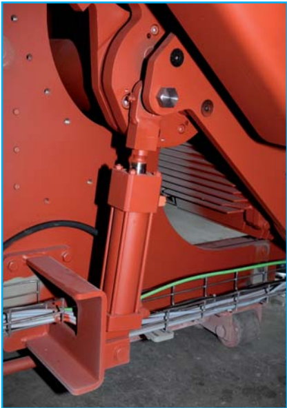
Fig. 6: Height adjustment of saw shaft by a hydraulic cylinder
