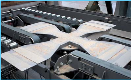
Fig. 21: Automatic panel turning unit
