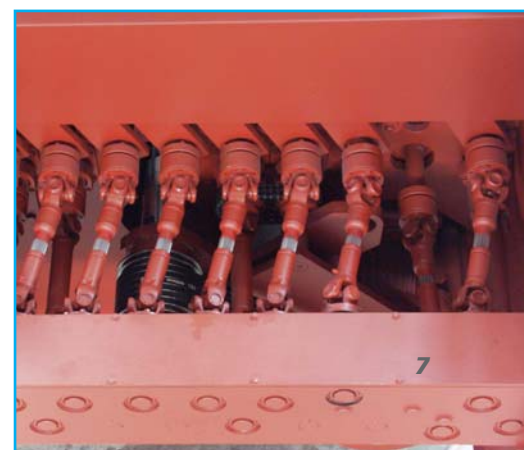
Fig. 18: Drive of feed rollers via cardan shafts
