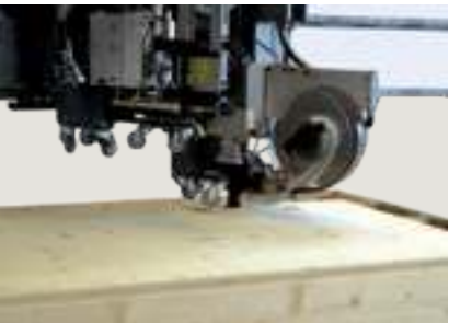
Nail pusher Using the nail impression unit also significantly increases the quality of fastening. One common area of application is the fastening of gypsum plasterboard. Speed: 1.25 sec/nail
