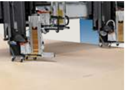
Parallel attachment The sheathing is secured in parallel with two identical fastening units. Up to 40% higher performance can be achieved.
