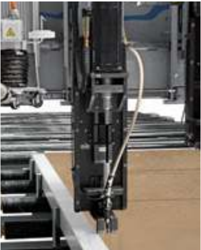
Screws Fastening with screws suited for gypsum plasterboard or assembly panels. Only approx. 2.5 seconds are required per screw.
