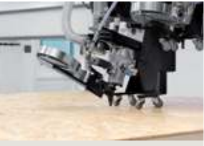
Swiveling units for nailing devices ▪ Swiveling unit for meeting the correct edge clearances, for example in the case of narrow studs or 2" x 4" construction method ▪ Horizontal swiveling to correctly attach soft wood fiber panels
