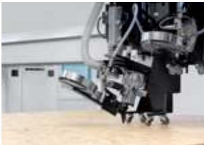
Option: swiveling chuck for nailing devices
