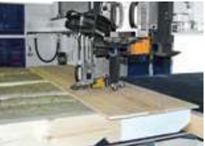
Fastening shuttering boards The attachment devices also allow you to automatically fasten panels for eaves shuttering.
